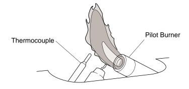
Figure 19 - Incorrect Pilot Flame Pattern
